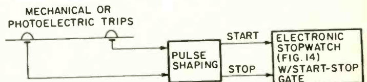
Fig. 17—Similarly, drag-strip speedometer measures time.
