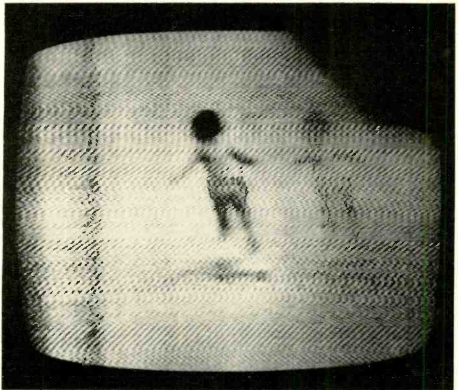
Fig. 1—Five faults show up in this TV picture. They include corner shadow, ghosts, dark vertical bars, adjacent-channel interference and poor focus. A sixth problem, blooming, became apparent when the brightness was turned up. A simple repair?
