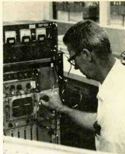
Troubleshooting a subcarrier oscillator.
